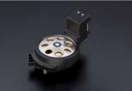
Motorized Seven Position Nosepiece/ U-D7REA Equipped with a DIC slider slot, this revolving nosepiece allows simultaneous attachment of seven objectives. It is especially suitable for continuous observations from low to high magnifications and combining specific objectives, such as polarized light observations.
