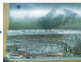
Upper-portion illumination of surface fracture (metal)
